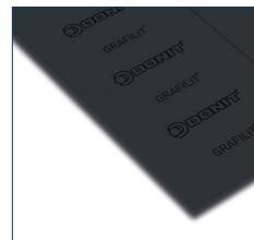
GRAFILIT® EM is an expanded graphite based material with expanded stainless steel insert, which enables applications with high operation pressures, including cycling operations. Even surface pressure distribution on gasket provides excellent thermomechanical properties and sealing characteristics, and increase blowout resistance. Therefore material is particularly suitable for high temperature applications in petrochemical industry and steam supply.
